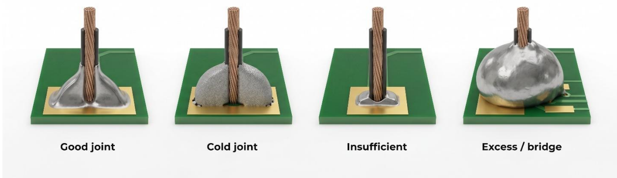
Figure 1. Inspect the shape and wetting of each solder joint. Do not judge joint quality only by surface brightness, because lead-free solder may appear dull even when properly soldered.
