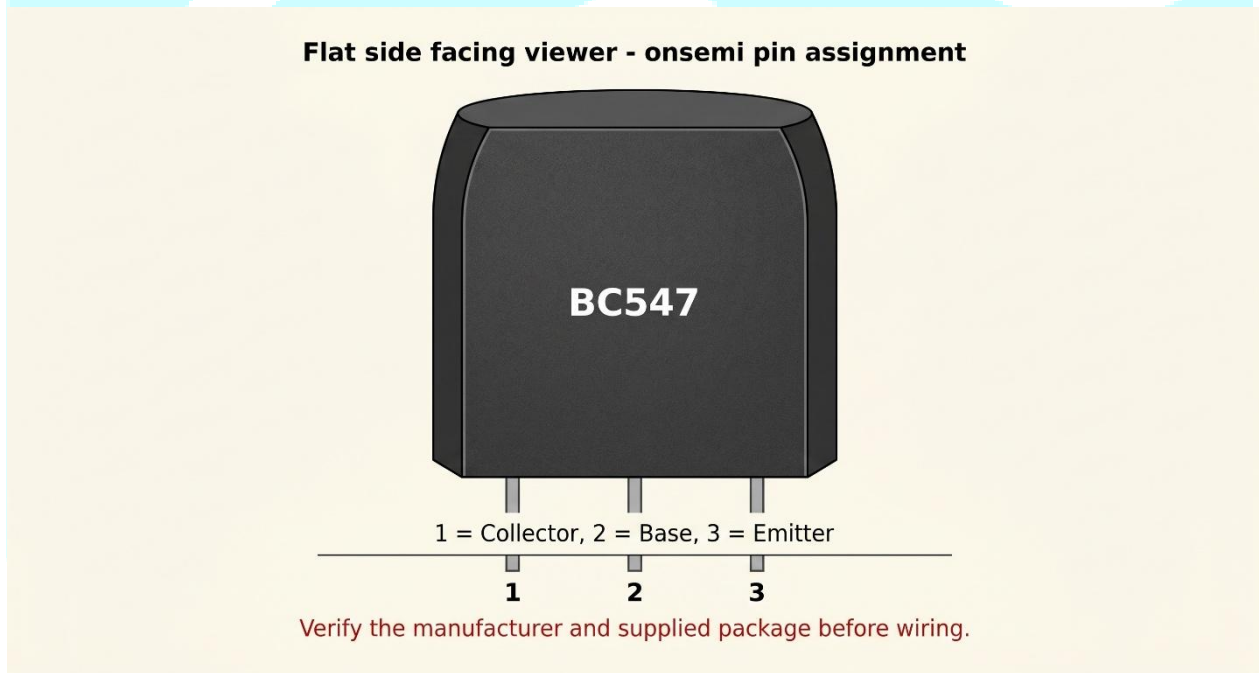
Figure 1. onsemi BC547 TO-92 pin assignment, flat side facing the viewer. Confirm the manufacturer of the supplied part.
